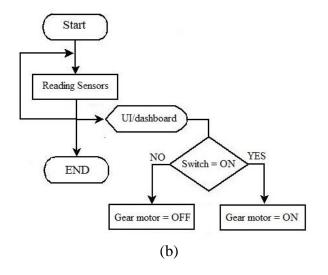
Fig. 4 The flowchart of system software (a) Data monitoring and temperature control (b) Feed level monitoring and feeding control.
